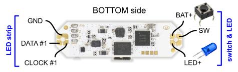
Connect a LED diode (forward voltage: 1.7-3.3V) between the **LED+** and any **GND** pad to get an external battery charging indication.
