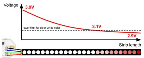
This problem starts to show with LED digital strips as short as 100-150 pixels. To combat the inevitable voltage drop, run parallel power cables of sufficient thickness (>0.5mm²/22AWG) from the **VCC** and **GND** pads of the FT2 chip and connect them to the digital LED strip at several spots along its total run length:
