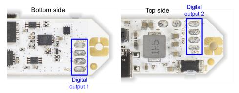
The FT2 chip has 2 sets of digital outputs, one from each side of the board. By default, the digital output #2 mirrors the functionality of the digital output #1 and come preconfigured as follows:
