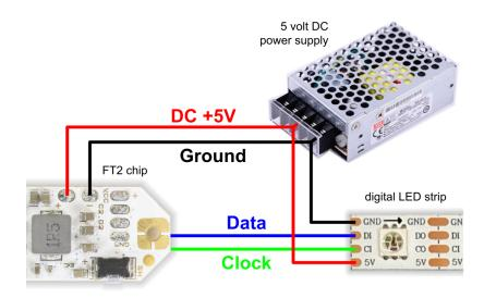
Note: In this configuration the voltage converter is not used, so it doesn't matter if it is bypassed or not.
